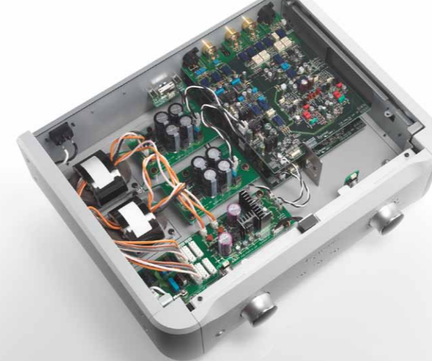
Highly rigid thick aluminum enclosure and internal construction
